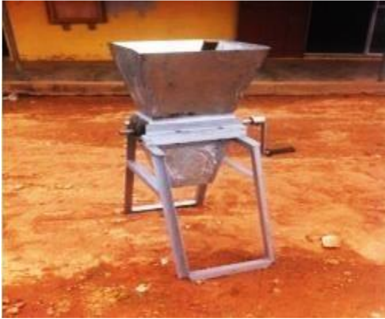
Figure 2.3: The constructed hand-operated manual cassava grater (Apodi et al., 2018)
