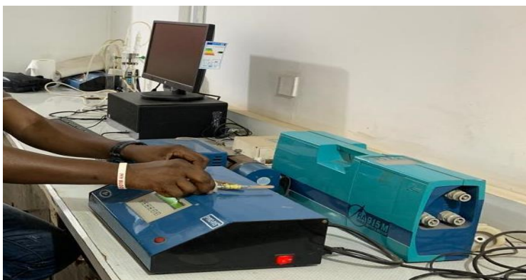
Plate 3.2: PYRO-915+ and RA 915 M, Mercury Analyzer (SHEATHE Lab, KNUST)
