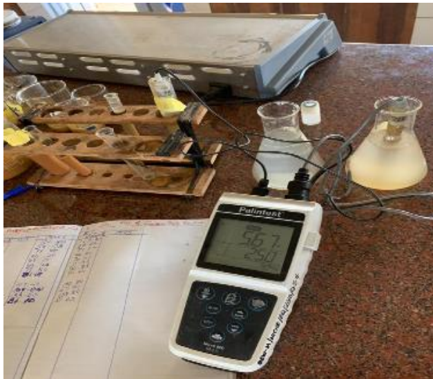
Plate 3.3. Hanna H28116731 DiSt-6 EC meter: Hach H550 Rugged Pocket pH meter
