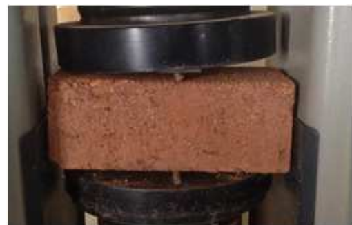
Figure 6: Set-up of tensile strength test.
