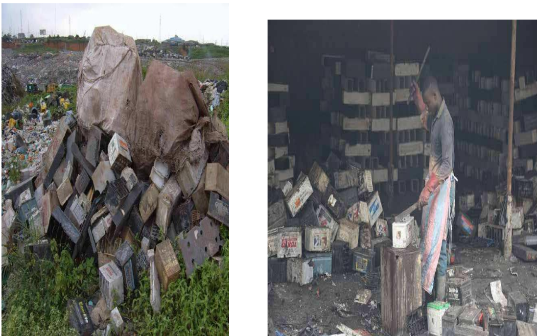
Figure 2.3: Opening of drained lead-acid batteries (Left) and Empty battery-cases (Right). Source: Oeko-Institute (2014)
