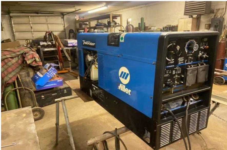
Figure 3.12: Miller Electric Welding Machine used for the arc welding process.
