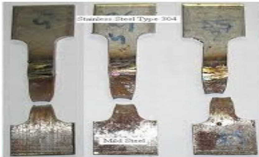
Figure 3.16: HAZ Sample test specimens for tensile testing
