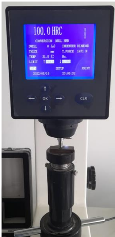
Figure 3.12: Digital B Rockwell Hardness Testing Machine.
