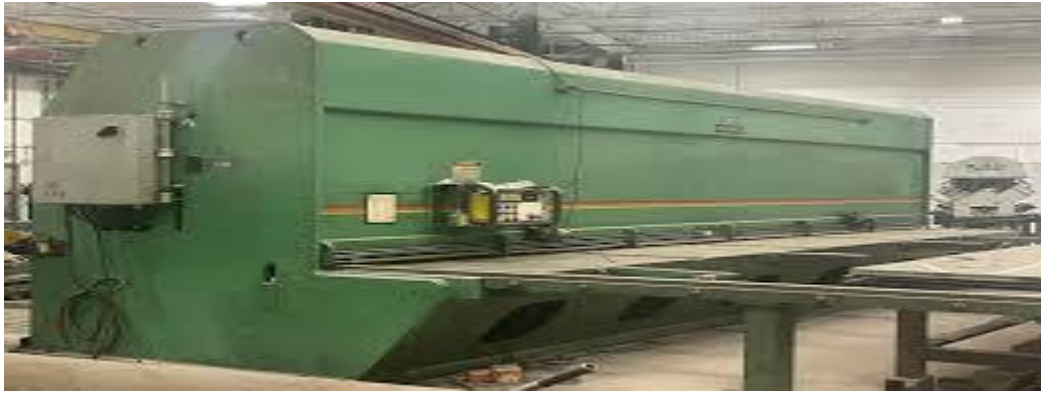
Figure 3.11: Accurshear Power Cutting Machine for cutting plate
