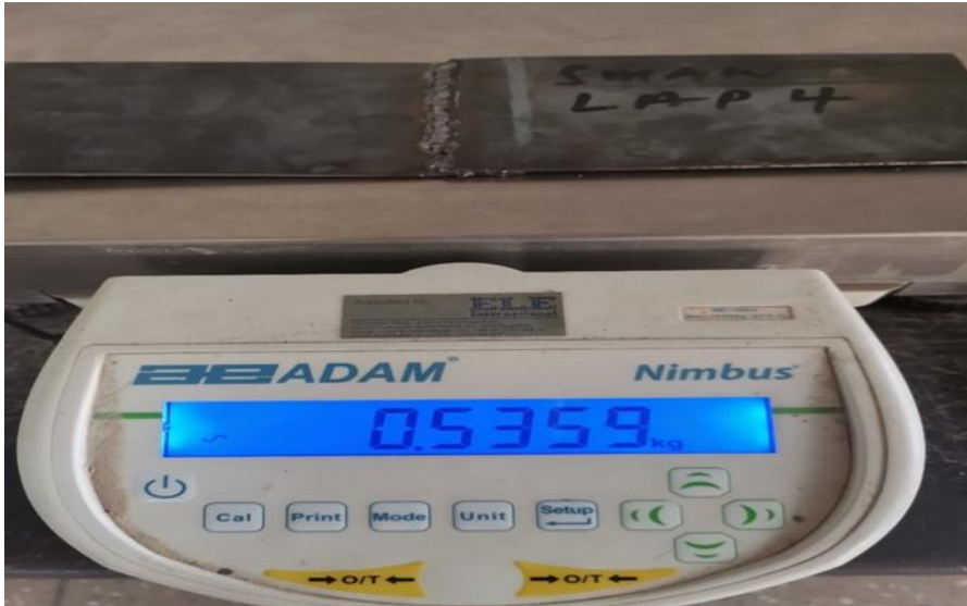
Figure 3.17: Digital balance was used to take mass samples before and after testing
