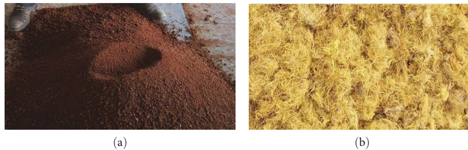
FIGURE 1: Raw materials: (a) sieved laterite ready for use and (b) sample palm nut fibres.
