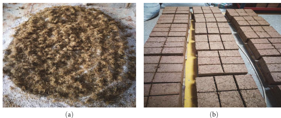
FIGURE 2: Preparation of brick specimens: (a) mixing of mortar and (b) air drying of brick specimens.
