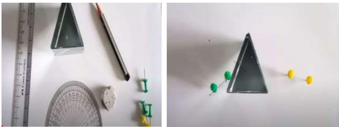
Figure 4.3: Experimental setup for verification of Snell's law
