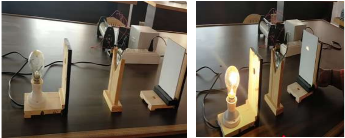
Figure 4.5: Experimental setup to determine the focal length of a concave mirror
