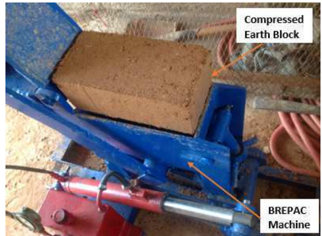
Figure 1. Moulding of Block with BREPAC Machine.
