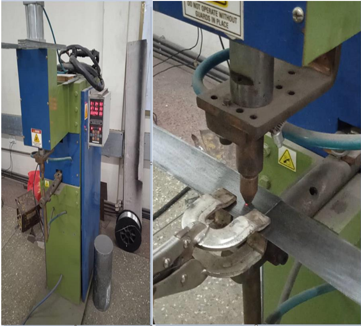
Figure 2 Spot Welding of Mild Steel
