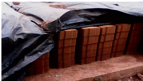
Figure 4: Curing of the specimen with water and polythene sheets.
