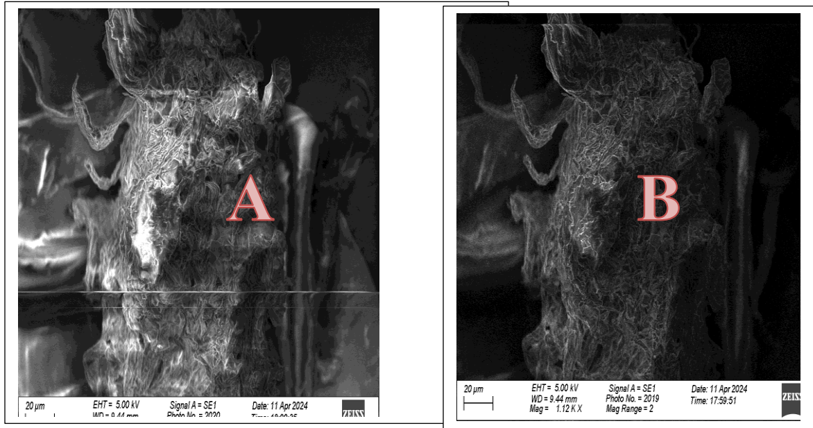
Figure 4.1: SEM micrograph of the extracted MSM-MCC
