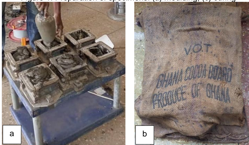
Figure 1. Preparation of specimens: (a) moulding, (c) curing
