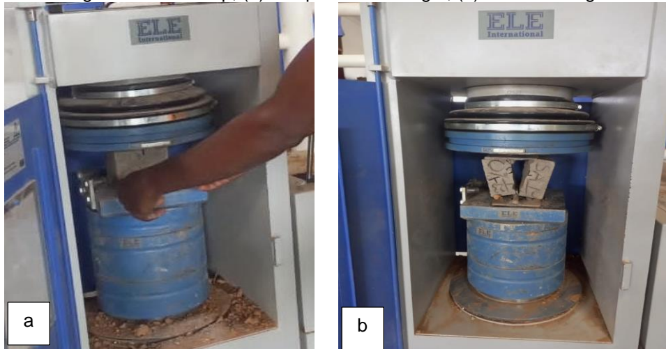
Figure 2: Test setup, (a) compressive strength, (b) tensile strength
