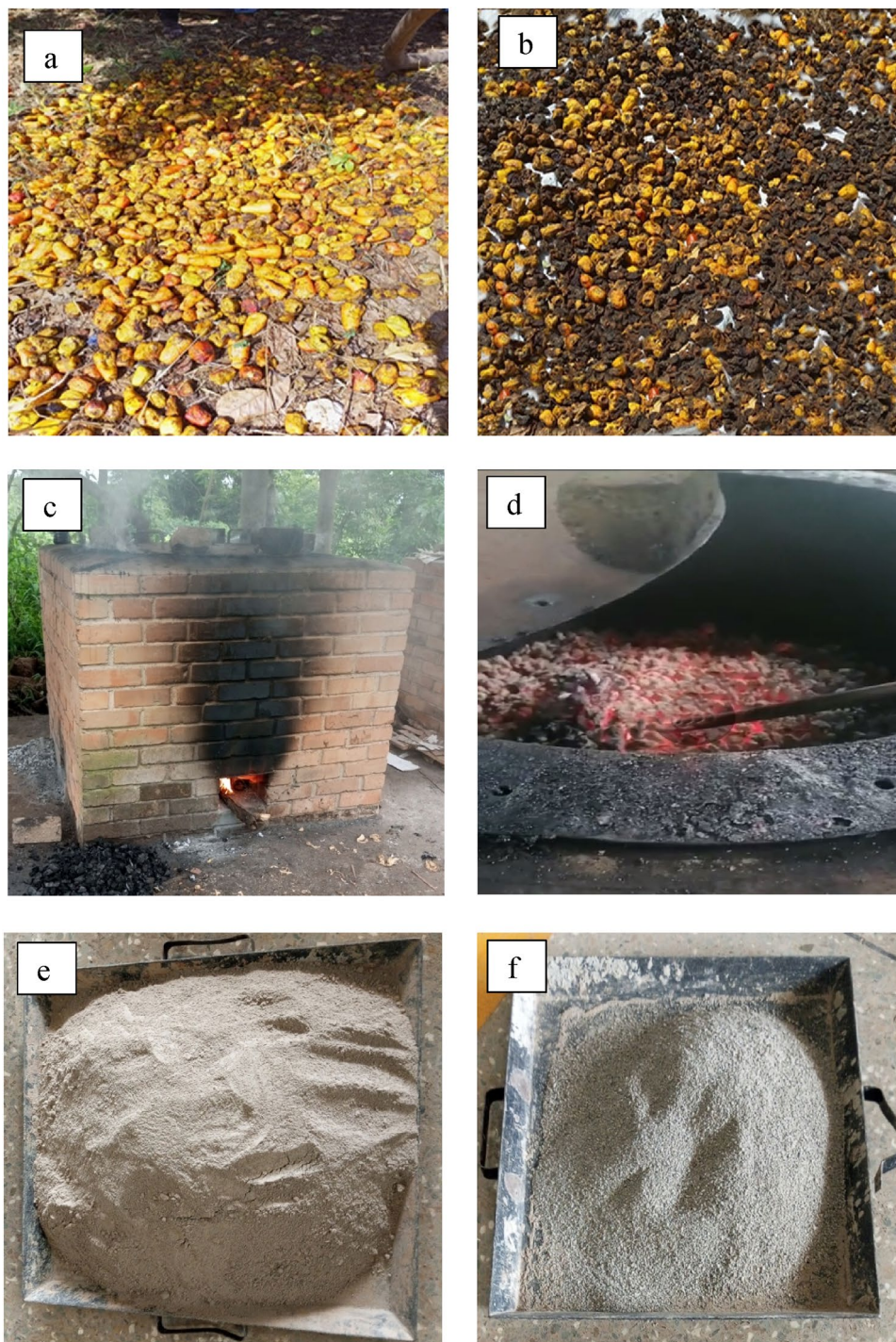
Figure 1. Production process of cashew apple ash: (a) cashew apple waste, (b) sun-drying of cashew apple waste, (c) burning of cashew apple waste in a locally built furnace, (d) burning of cashew apple waste at temperature of 735 °C, (e) cashew apple ash ground into fine particles, (f) sieved cashew apple ash.
