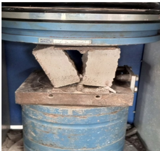
Figure 4. Split block specimen under tensile strength test.
