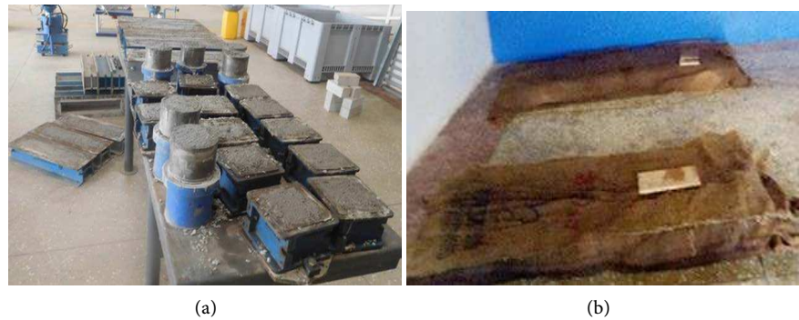
Figure 2. Preparation of concrete specimens at the laboratory. (a) Moulding of concrete specimens; (b) Wet jute sack curing of concrete specimens.
