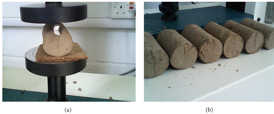
FIGURE 5: (a) Specimen under tensile stress, (b) failed specimen.
