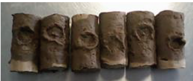
FIGURE 6: Drip test specimen showing depth of pit.
