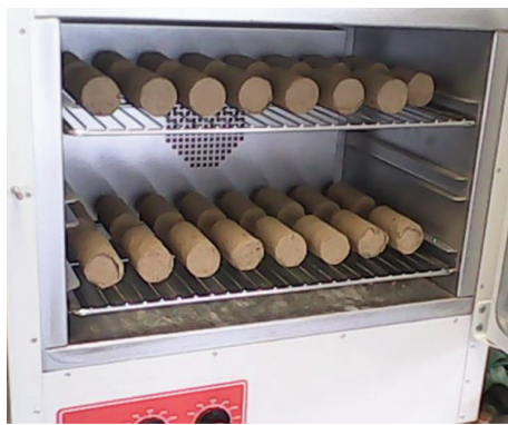
FIGURE 3: Drying specimen in oven.
