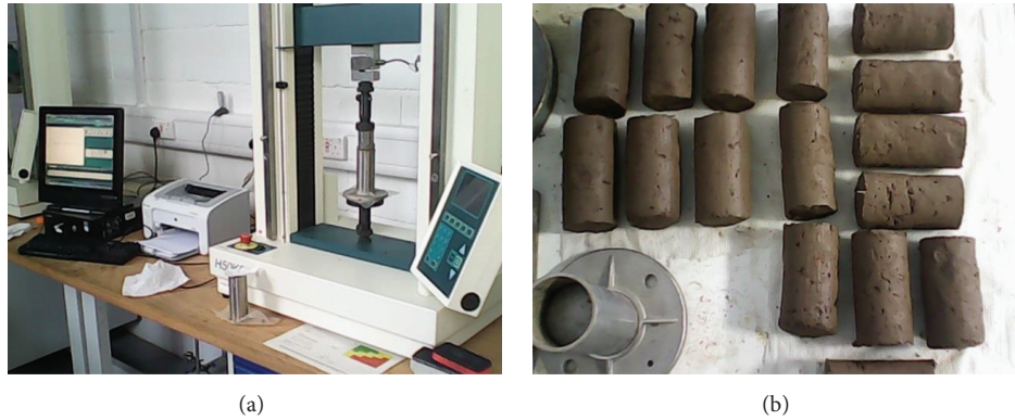
FIGURE 2: (a) Specimen under compaction, (b) specimen extruded from mould.
