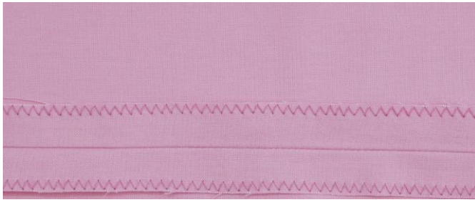
Plate 1: Zigzag stitch used as a seam finish
