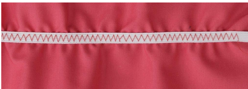
Plate 3: Zigzag stitch used to attach Insert elastic
