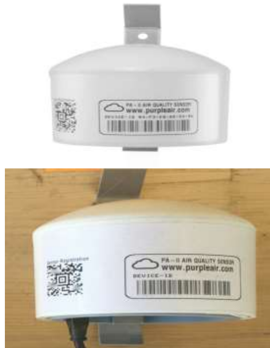
Figure 3.2: PurpleAir Classic (PA-II) Air Quality Monitor
