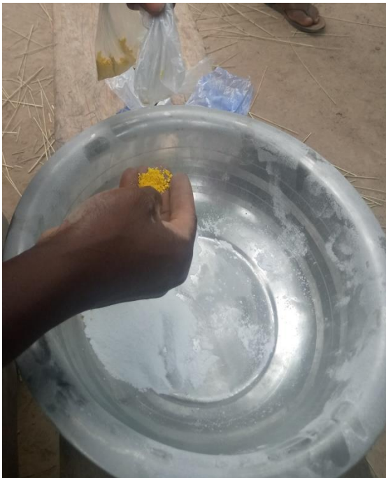
Figure 5.5 Adding powdered dye to the sieved glass and arranging it in the mould.
