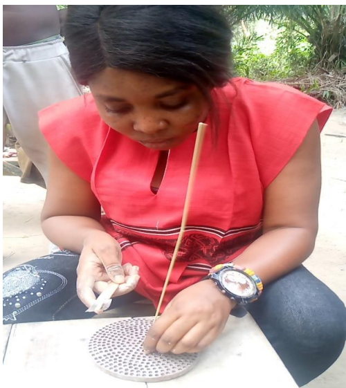
Figure 5.3 Filling portion of the mould with bamboo stick to create hole in the beads.
