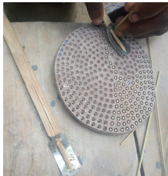
Figure 5.3 Filling portion of the mould with bamboo stick to create hole in the beads.
