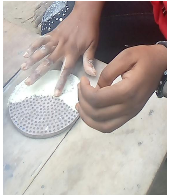
Figure 5.5 Adding powdered dye to the sieved glass and arranging it in the mould.
