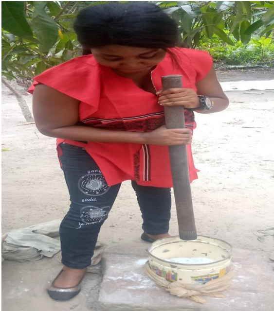
Figure 5.4 Crushing bottles with metal pistil and mortar and sieving of crushed bottles.
