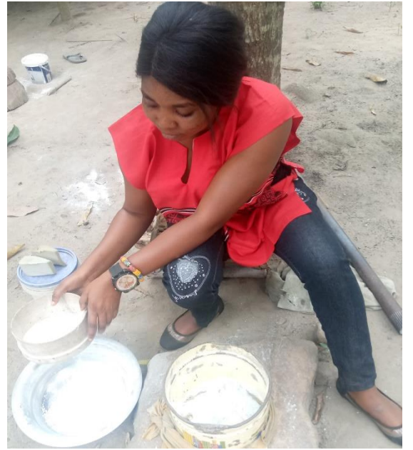
Figure 5.4 Crushing bottles with metal pistil and mortar and sieving of crushed bottles.
