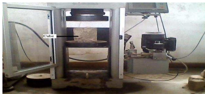
Figure 3: Concrete cube being crushed
