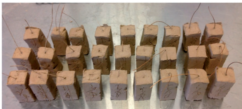
Figure 4. Drying samples for pull-out test.
