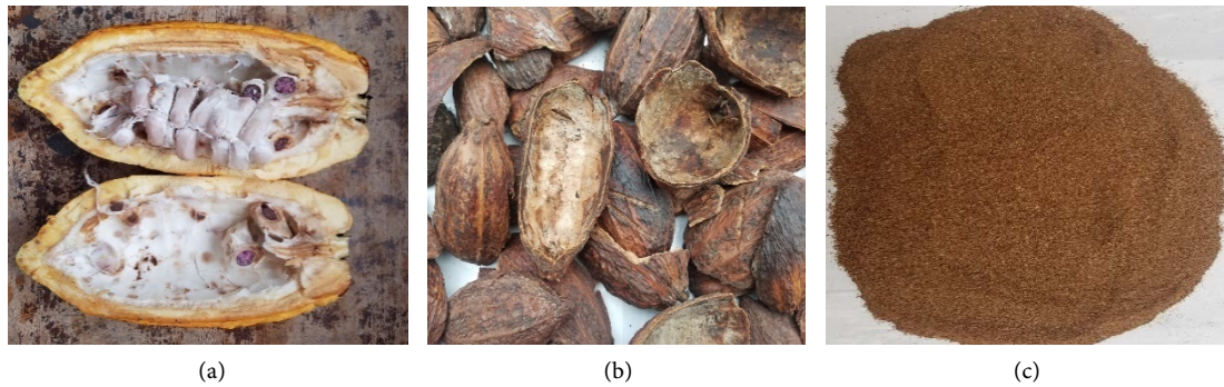
Figure 3. Stages of processing cacao pod into particles. (a) Fresh cacao pod; (b) Dried cacao pod; (c) Cocoa pod particles.
