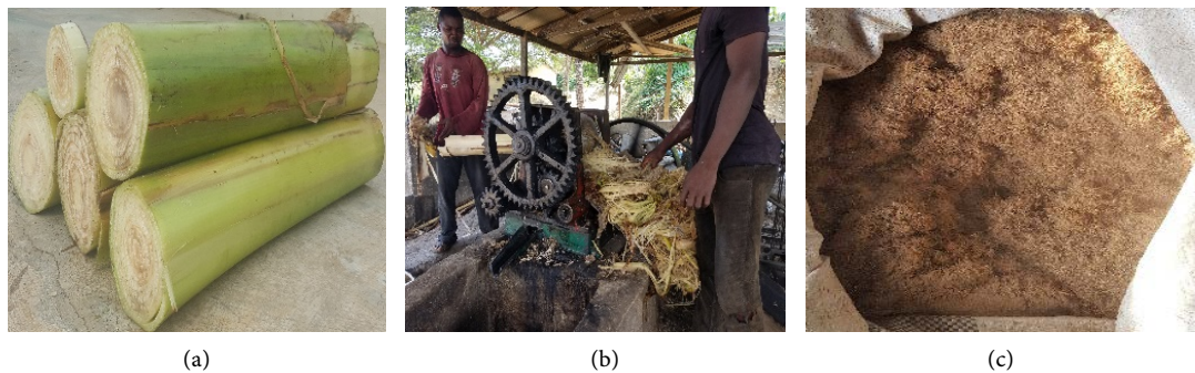
Figure 1. Stages of processing plantain pseudostem into particles. (a) Fresh plantain pseudostem ; (b) Water extraction from plantain pseudostem ; (c) Plantain pseudostem particles.
