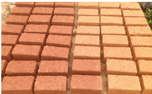
Fig. 3: Drying of enhanced soil blocks.
