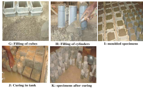
Plate B 3b Casting of moulds and curing
