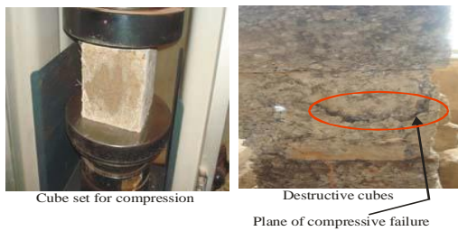
Plate B 3c Destructive cubes
